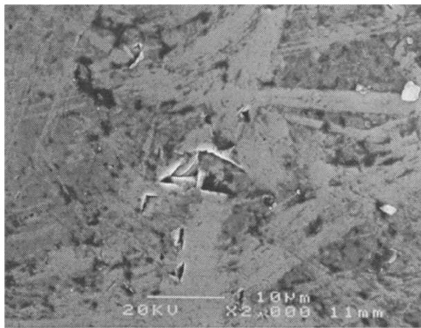
Fig. 3 Electron microscope photograph of the steel ball bearing surface at 10-μm scale.
